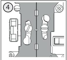
When combining multiple devices (e.g. socket and socket or switch) pay attention to the exact alignment. Take advantage of the notches to align the supporting frames.
