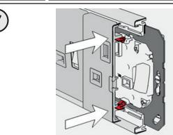
Press the design cover evenly on the socket insert. Take care, that you plug the spring terminals in the provided guides.
