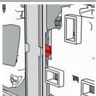
Do not use other screws than the enclosed screws of the wall box to install the inserts. When using other screws, design frame rests against the screw heads. (ref. No. SCREW-30 /-50 /-70)
