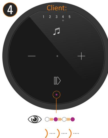
4. Wait until both devices have found each other. Then the A100 LED again shows the source with corresponding LED colour and the status LEDs on the A100 permanently show the pink LED - done.
