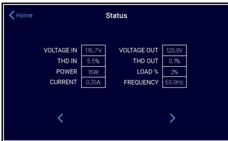
Here you can see the P15's overall performance data. Note how in the above image the THD output is significantly reduced and the output voltage is a stable 120 Volts. Press the Home button to return to the Home screen.
