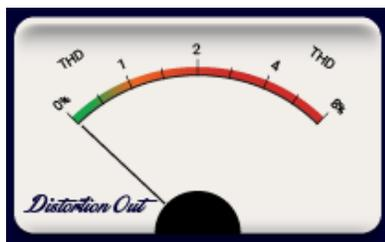
The Distortion Out is a measure of the THD (Total Harmonic Distortion) present in your AC output voltage.
