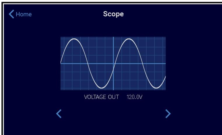
This is a fully functional oscilloscope that you can use to view the incoming AC waveform. Pressing either of the arrow buttons will scroll through the voltage in, voltage out and the difference windows. In this way you can see the degree to which the P15's output waveform is superior to the incoming AC sine wave.
