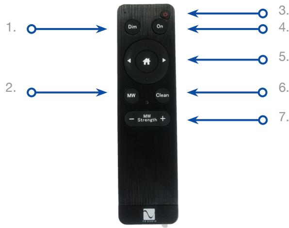
1. The Dim button turns the P15's display on and off.
