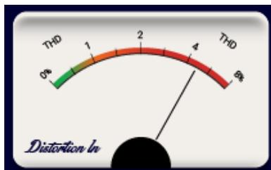
The Distortion In is a measure of the THD (Total Harmonic Distortion) present in your AC input voltage.
