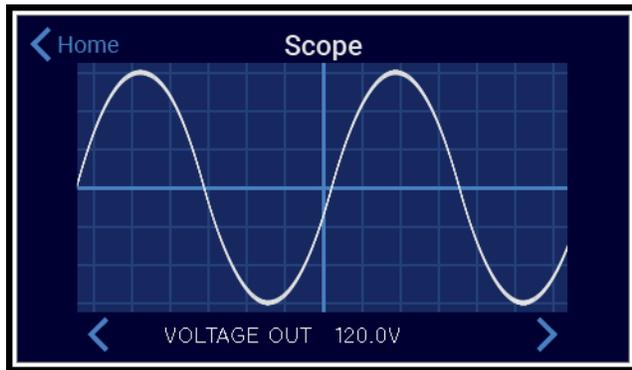
This is a fully functional oscilloscope that you can use to view the incoming AC waveform. Pressing either of the arrow buttons will scroll through the voltage in, voltage out and the difference windows. In this way you can see the degree to which the P12's output waveform is superior to the incoming AC Sine wave.
