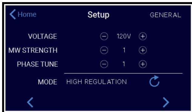
**Voltage** Here you can globally adjust the output voltage for the P12. Bear in mind that the P12 will output the same voltage from all zones. They are not individually adjustable.
