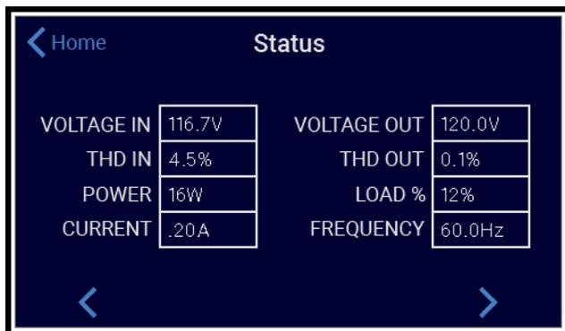
Here you can see the P12's overall performance data. Note how in the above image the THD output is significantly reduced and the output voltage is a stable 120 Volts. Press the Home button to return to the Home screen.
