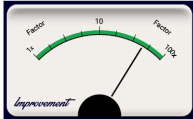
The Improvement Factor is an average of the voltage output and the THD output. It gives you a factor of how much the AC power is improved by the P12.
