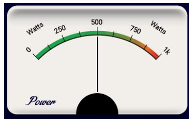
The Power Meter shows the total wattage output from the P12.
