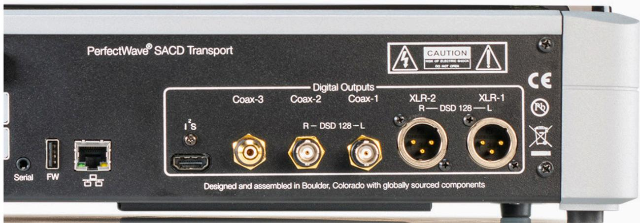
Although an HDMI cable is used for the I<sup>2</sup>S connections, it's important to note that I<sup>2</sup>S data is not HDMI data, and the PST's I<sup>2</sup>S output should not be connected to the HDMI input on a DAC or receiver. The HDMI connector and cabling are used only to deliver audio via I<sup>2</sup>S.
