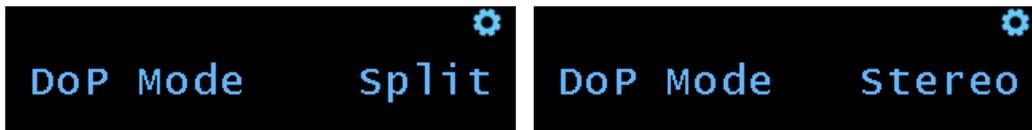
In “Stereo” mode, the DSD128 signal is encoded into a 352.8KHz PCM frame. The same signal is sent to all Coax and XLR connectors. However some DACs are not capable of decoding 352.8KHz frames. In “Split” mode, each channel (L and R) is encoded separately in a 176.4KHz PCM frame. The Left channel will be sent to the the “L” connectors and the Right channel will be sent to the “R” connectors. The Coax-3 output is always in stereo mode.
