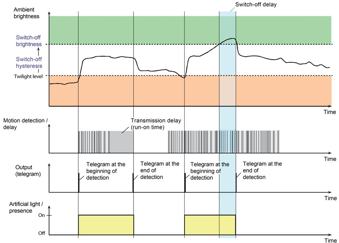
Figure 22: Brightness and motion evaluation with the presence detector
