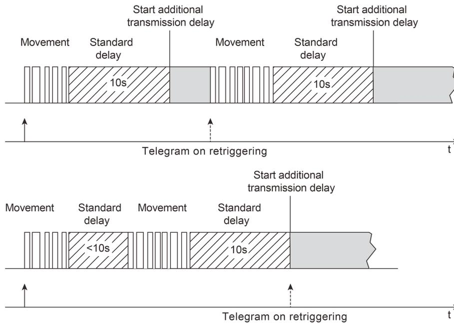
Figure 37: Triggering of a telegram when retriggering
