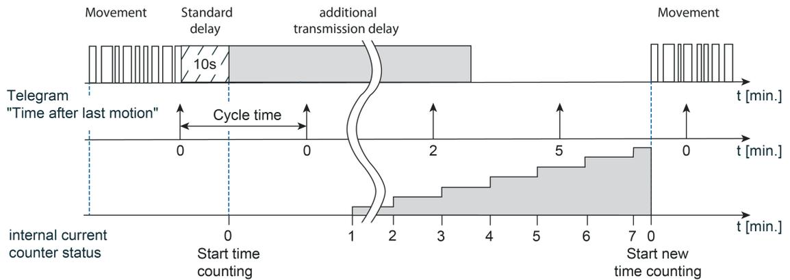
Figure 41: Measurement of the time period after last motion
