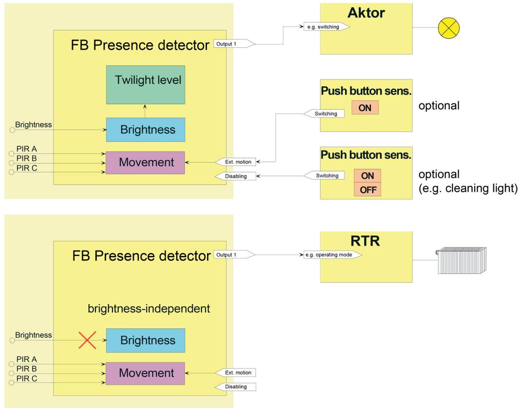
Figure 21: Application examples of the application presence detector
