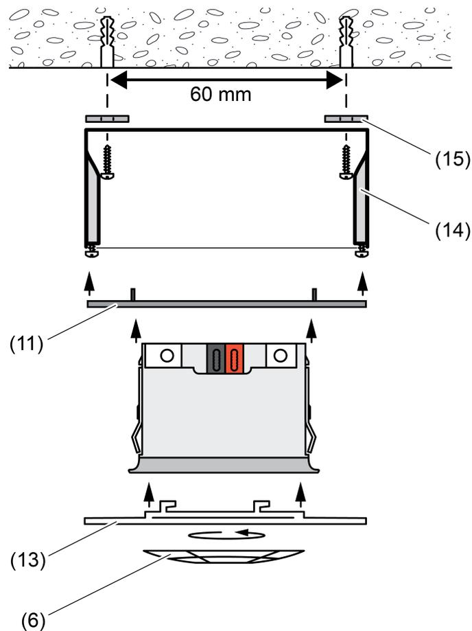
Figure 11: Mounting in the flush-mounted housing (accessories)
