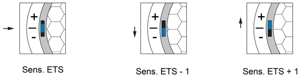
Figure 15: Adjustment ranges of the sensitivity adjuster on the device (-1 ↔ 0 ↔ +1)
