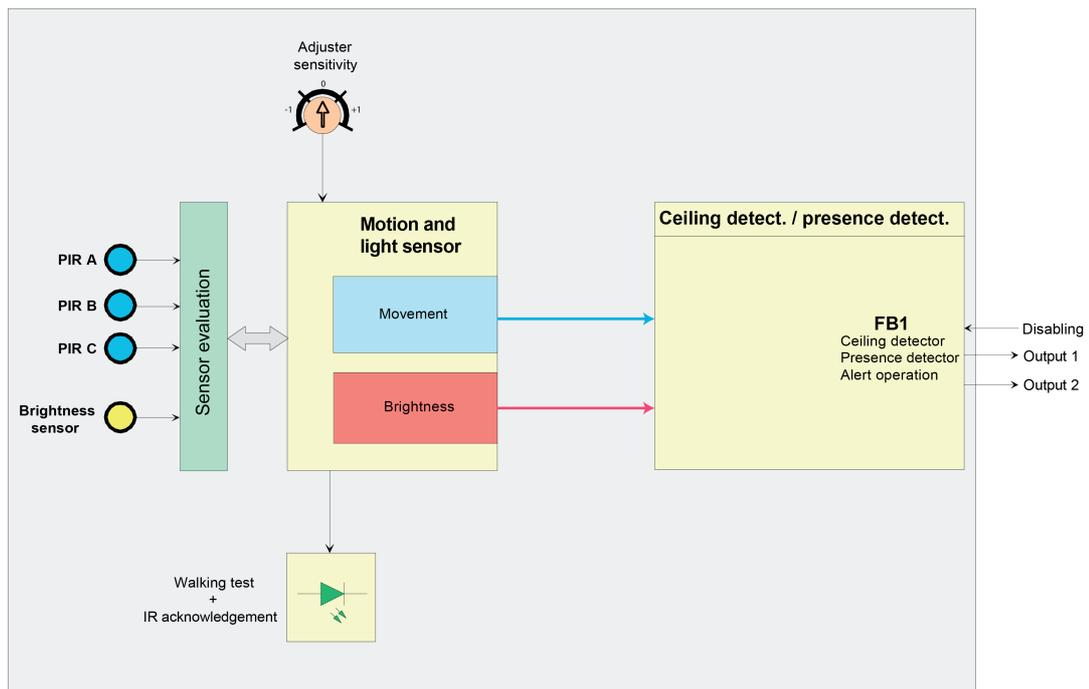
Figure 14: Block diagram of all device functions
