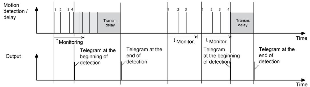
Figure 23: Motion evaluation with the detector
