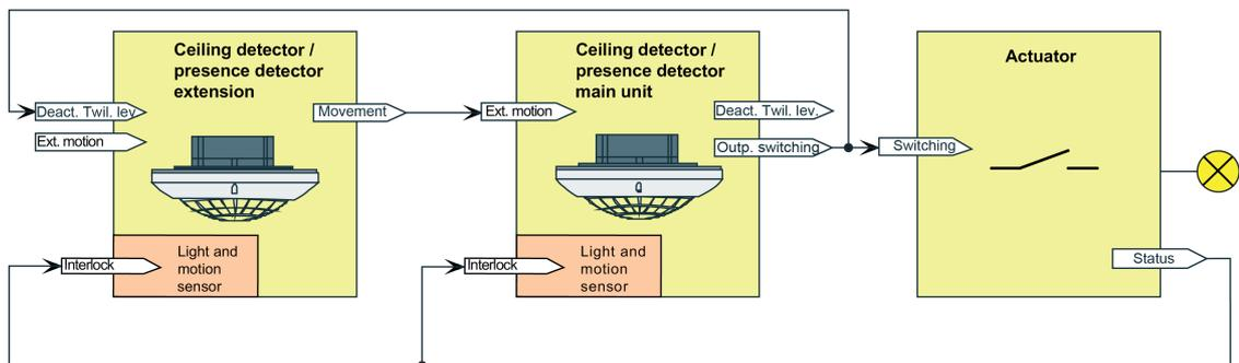
Figure 31: Application example with twilight level evaluation in the main unit and extensions for the data format "Switching"
