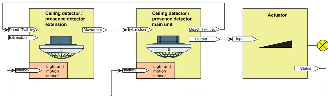
Figure 32: Application example with twilight level evaluation in the main unit and extensions
