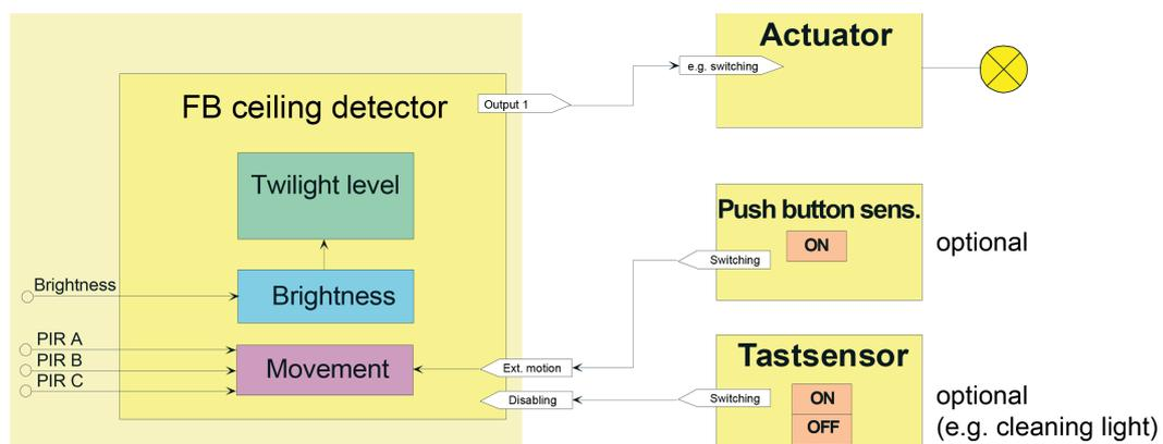
Figure 19: Application example of the application ceiling detector
