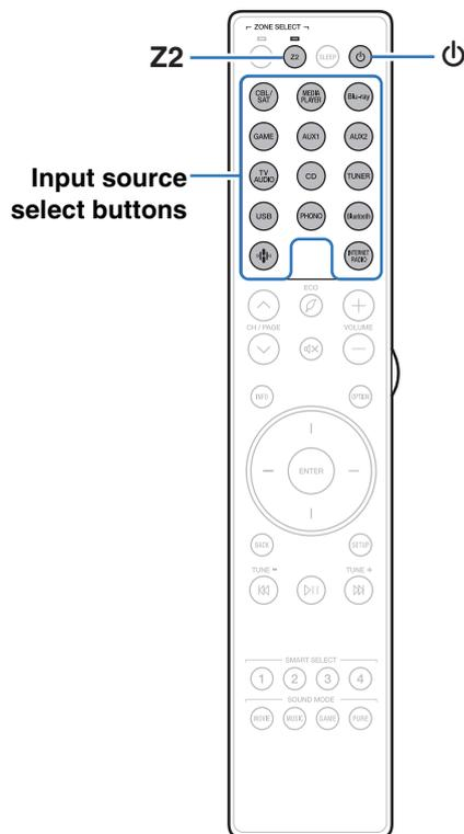
**1** Press Z2 to set the operating zone to ZONE2 with the remote control.
