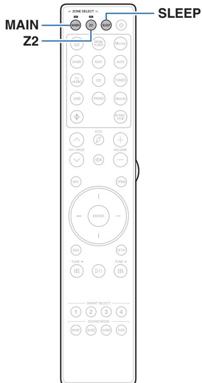
You can have the power automatically switched to standby once a set time has elapsed. This is convenient for viewing and listening while going to sleep. The sleep timer function can be set for each zone.
