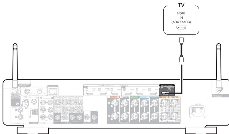
\* For 4K TVs we recommend using an HDMI cable labeled “High Speed” and “with Ethernet”.
