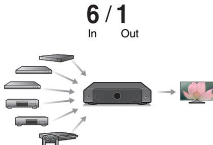
This unit is equipped with 6 HDMI inputs and 1 HDMI output enabling connection to various HDMI compatible devices such as Blu-ray Disc players, game consoles and HD video camcorders.
