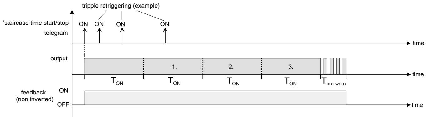
Fig. 14: Time extension for staircase lighting function
