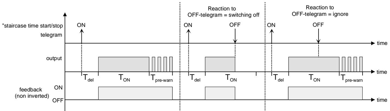
Fig. 12: Switch-off behaviour of the staircase function
