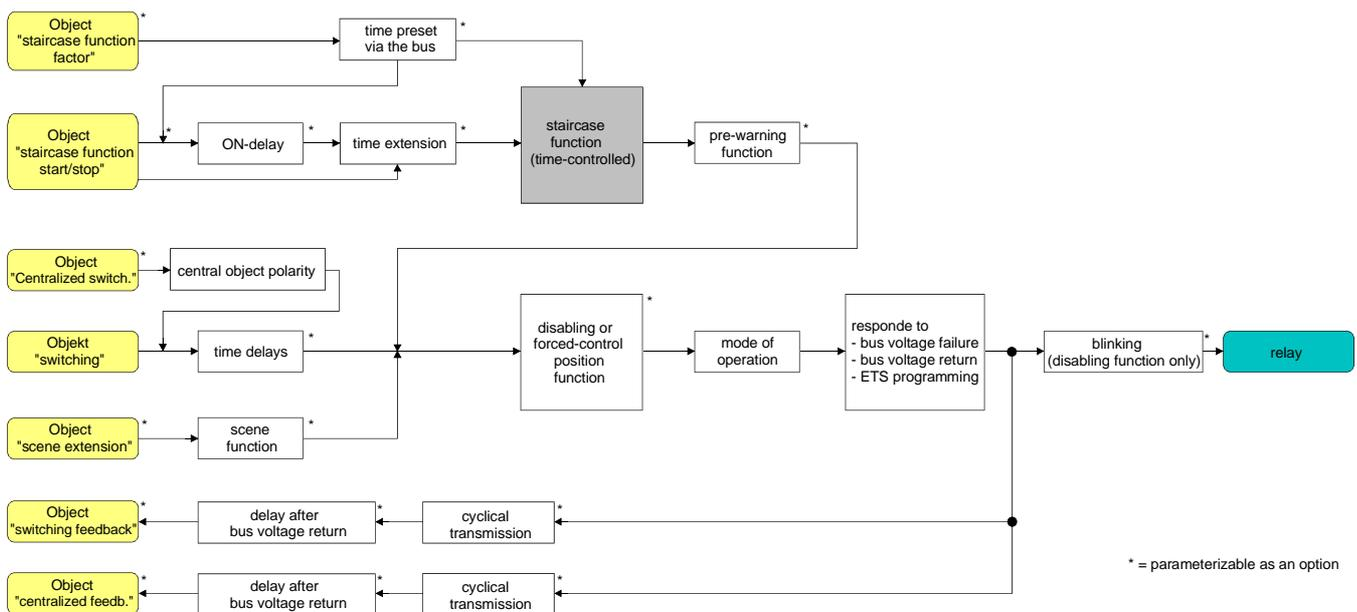
Fig. 10: Functional diagram of the staircase function
