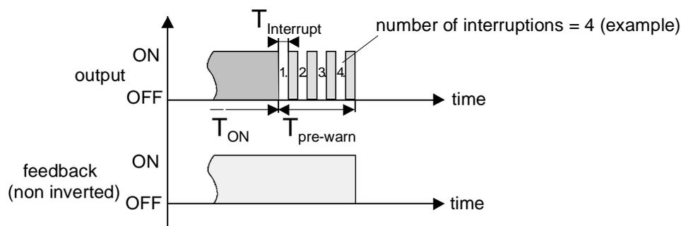
Fig.13: The pre-warning function of the staircase function
