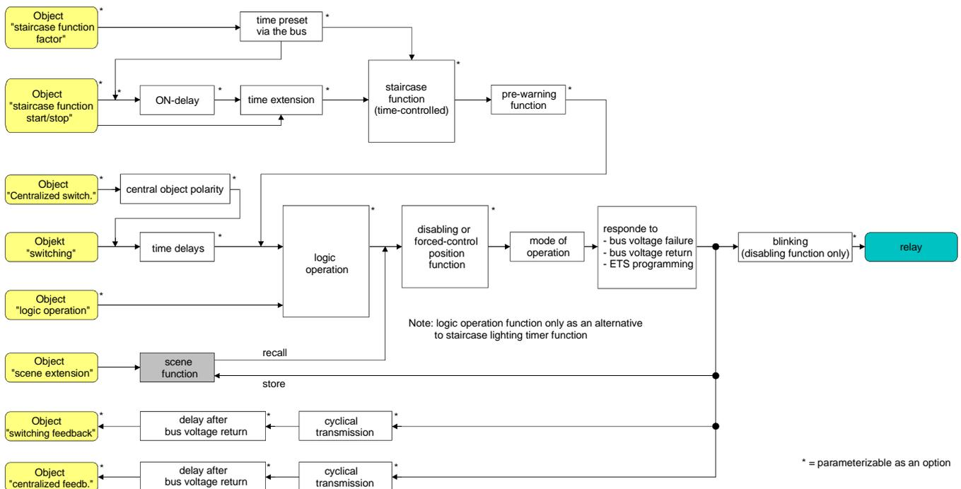
Fig. 15: Functional diagram of the scene function
