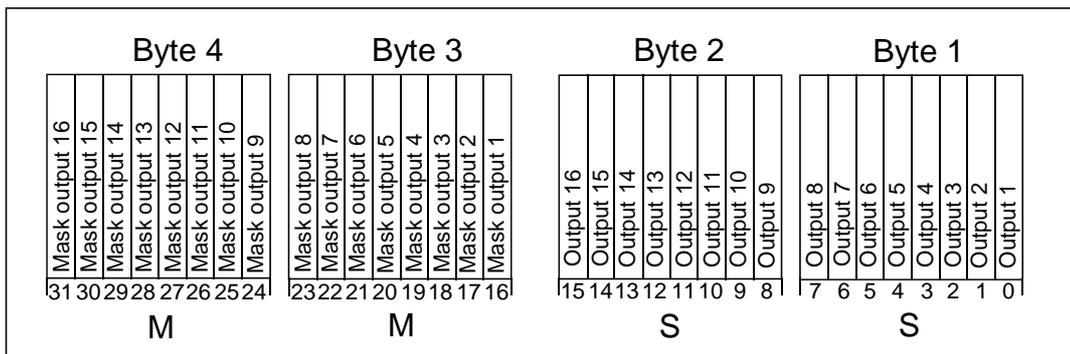
Fig. 5: Structure of the centralized feedback object
