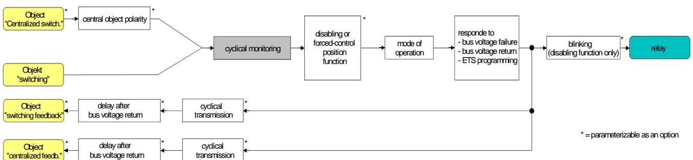
Fig. 8: Functional diagram of cyclical monitoring function
