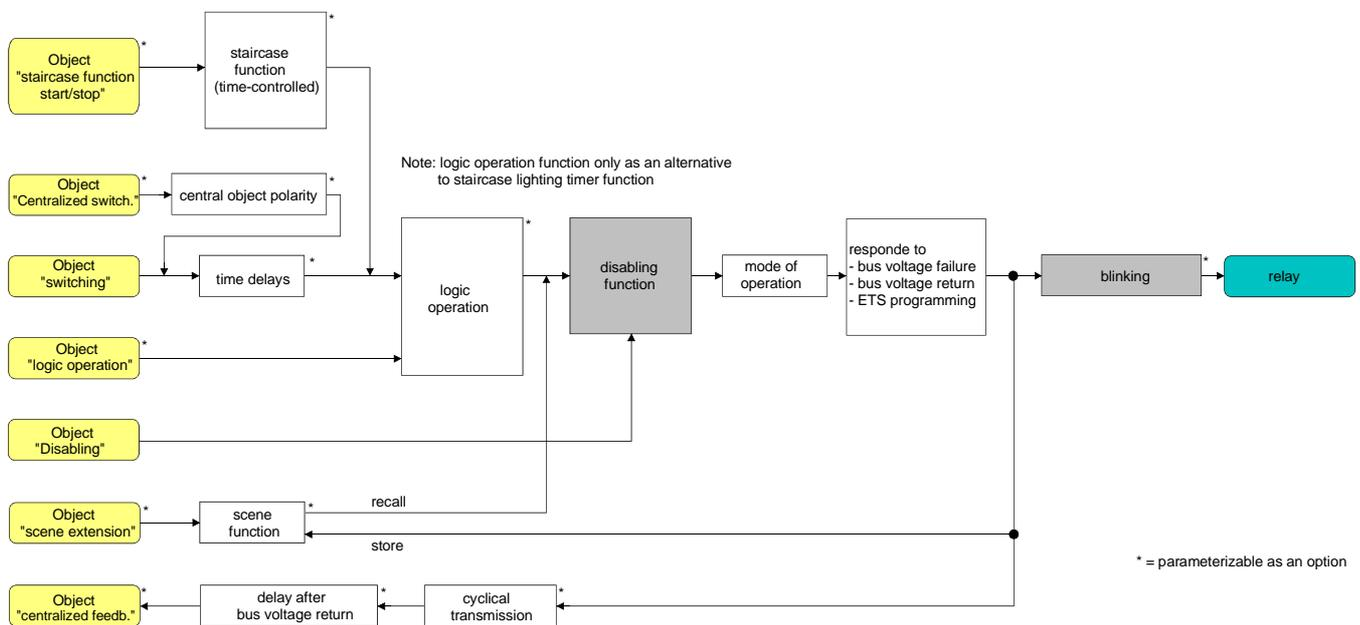
Fig. 19: Functional diagram of the disabling function
