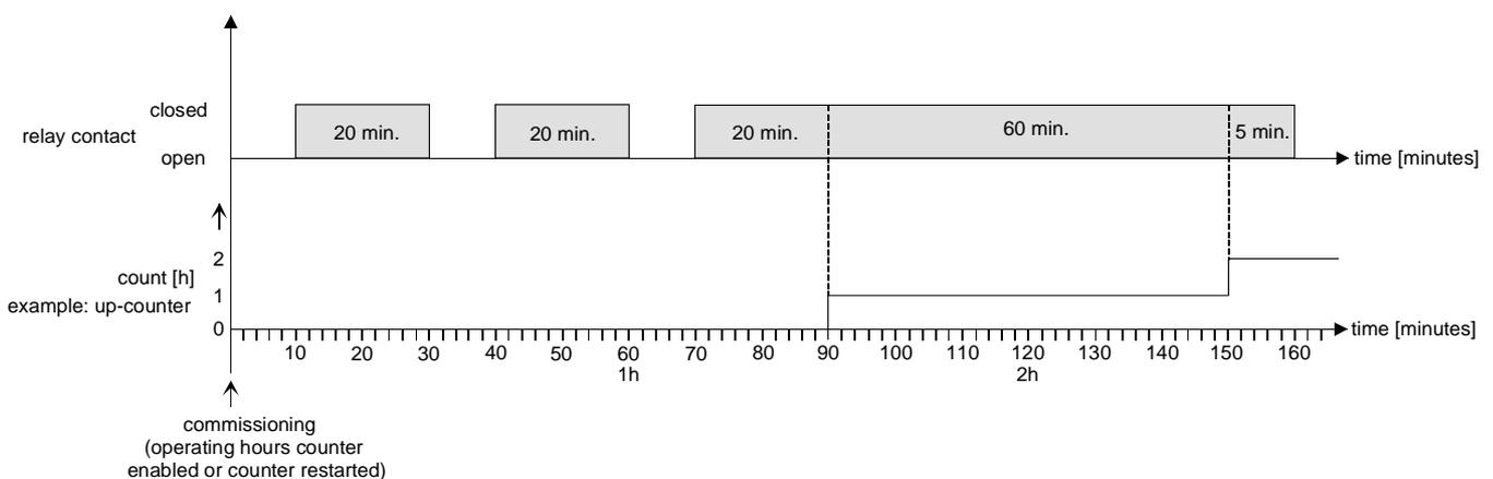
Fig. 16: Functional principle of the operating hours counter
