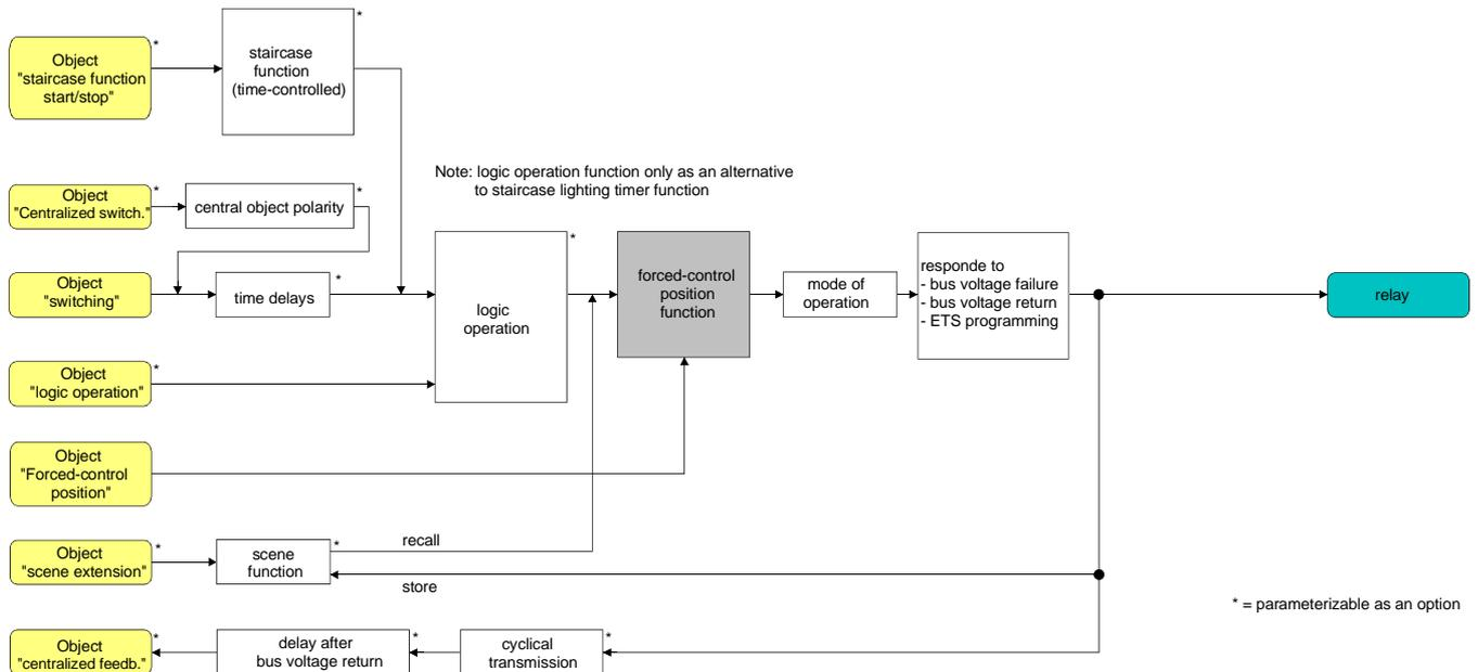
Fig. 20: Functional diagram of the forced-control position function
