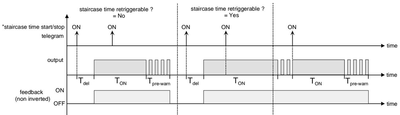
Fig. 11: Switch-on behaviour of the staircase function
