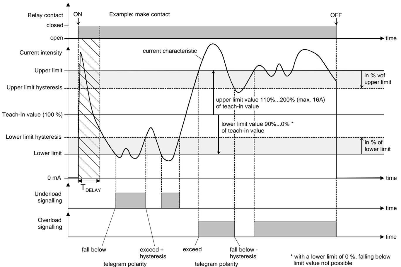
Fig. 18: Load monitoring with teach-in (exemplary current characteristic)
