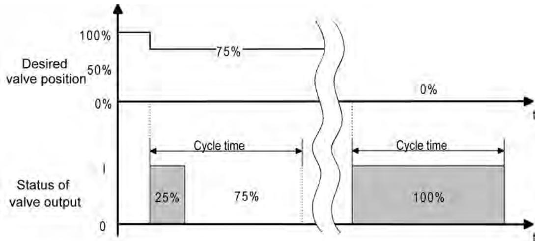
Figure 54: Conversion of a constant valve nominal position into an output signal with valve drives that are open when deenergized (example)
