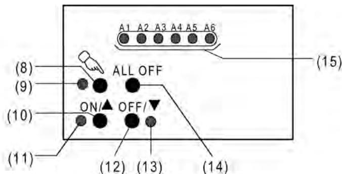
Figure 7: Controls and indicators for manual control on the front panel of the device.
