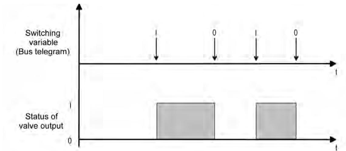
Figure 51: Conversion of a switching command value into an output signal with valve drives that are closed when deenergized (example)
