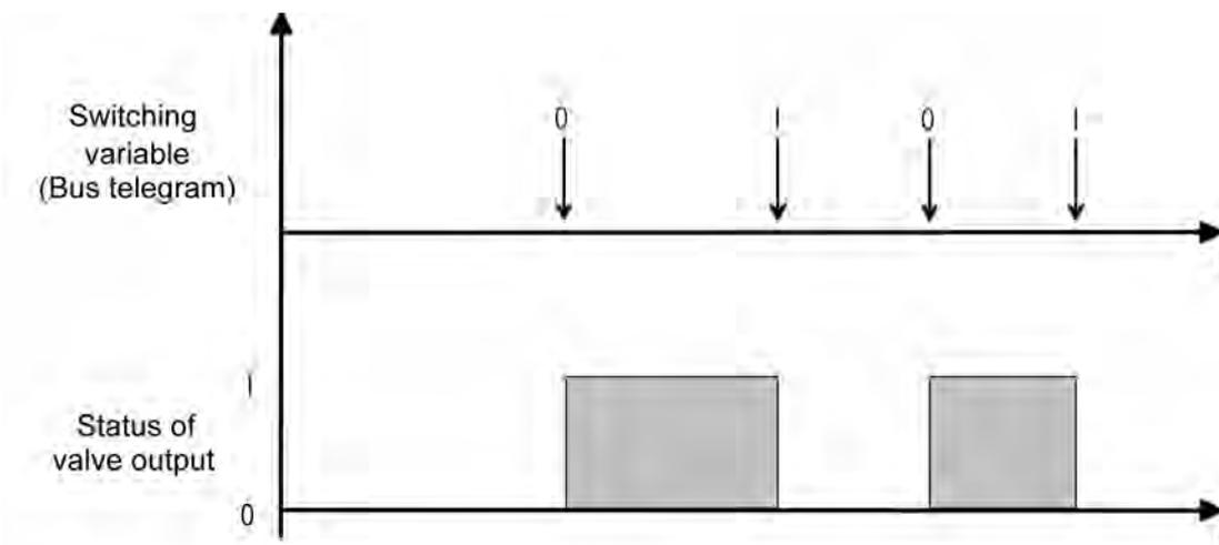
Figure 53: Conversion of a switching command value into an output signal with valve drives that are open when deenergized (example)
