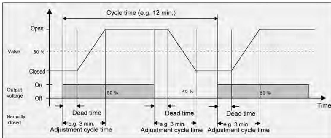
Figure 65: Idealised curve of the valve stroke: example for a command value of approx. 60 % for a valve closed when deenergized
