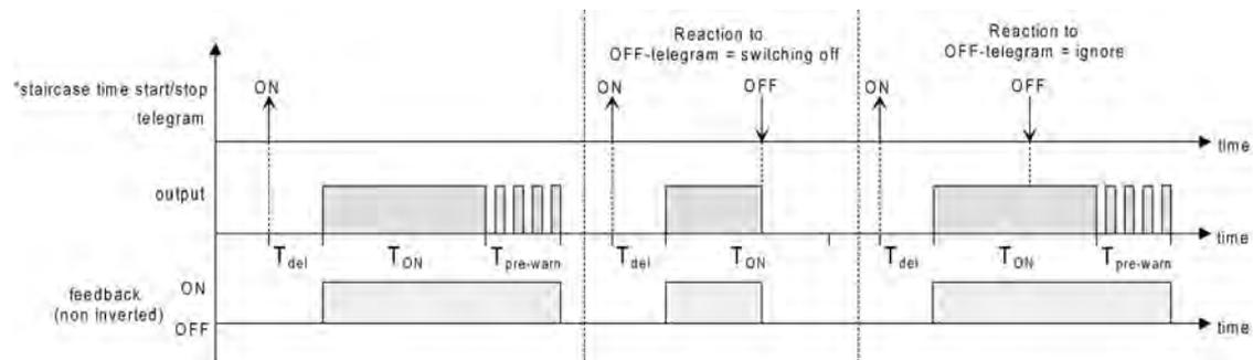
Figure 19: Switch-off behaviour of the staircase function
