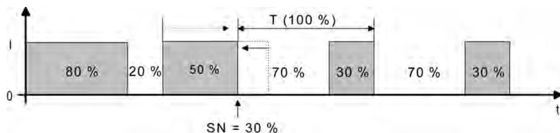
Figure 61: Command value change e.g. from 80 % to 30 % during the opening phase of the valve (opening phase too long)
