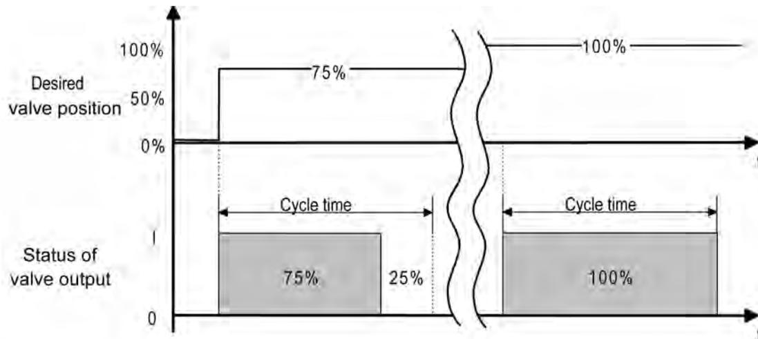
Figure 52: Conversion of a constant valve nominal position into an output signal with valve drives that are closed when deenergized (example)
