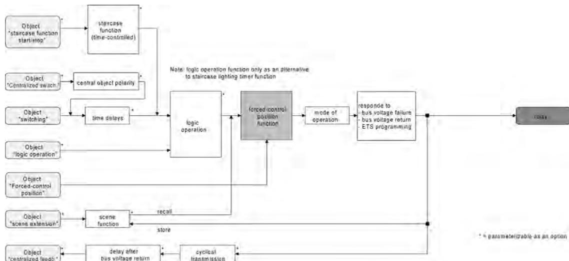
Figure 25: Functional diagram of the forced position function
