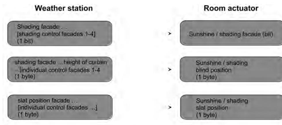
Figure 46: Programming of the communication objects for application example IV
