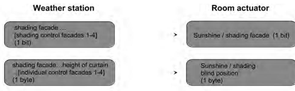
Figure 47: Programming of the communication objects for application example V
