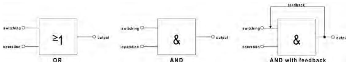
Figure 27: Gating operations of the logic function
