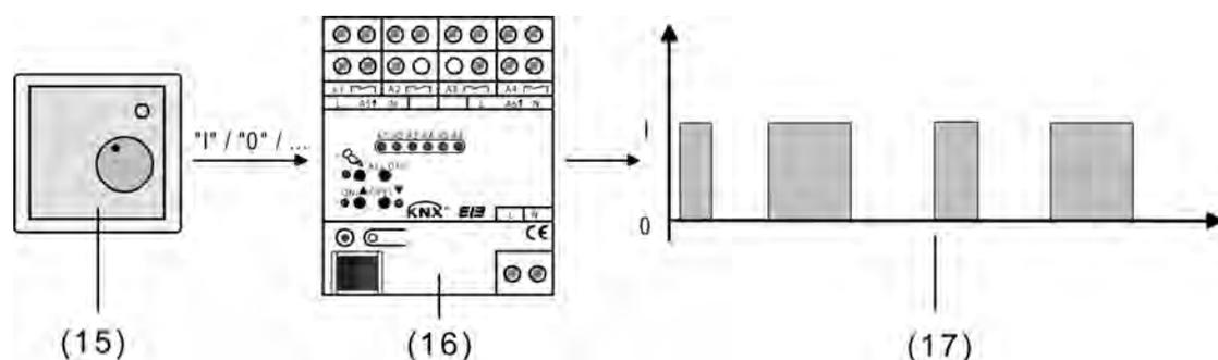
Figure 56: Command value principle with switching command value
