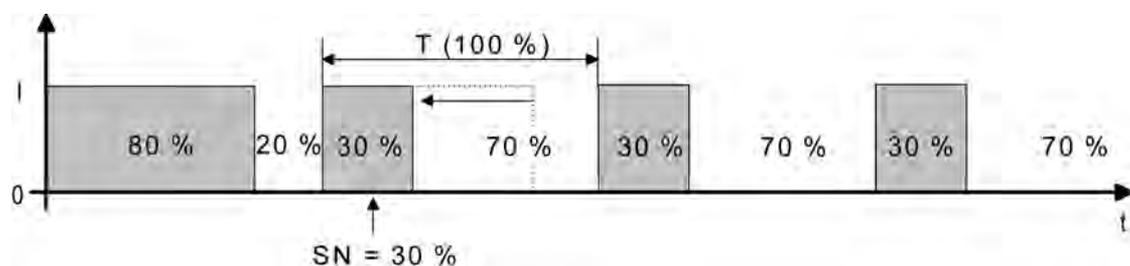
Figure 59: Command value change e.g. from 80 % to 30 % during the opening phase of the valve
