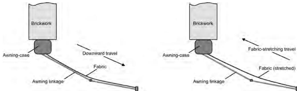
Figure 50: Fabric-stretching in an awning
