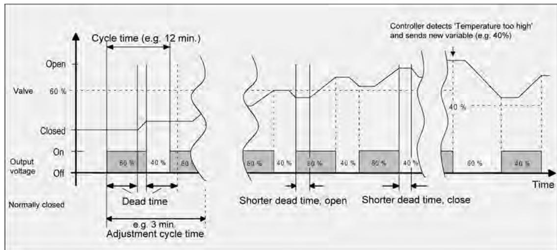
Figure 66: Idealised curve of the valve stroke: example for an initial command value of approx. 60 % for a valve closed when deenergized
