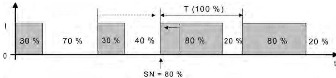
Figure 64: Command value change e.g. from 30 % to 80 % during the closing phase of the valve (closing phase too long)
