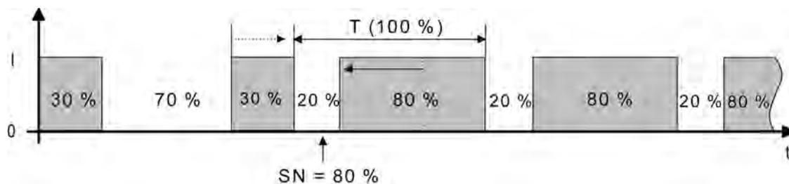
Figure 63: Command value change e.g. from 30 % to 80 % during the closing phase of the valve
