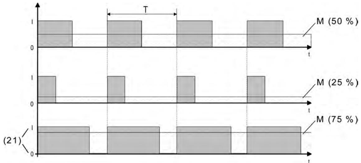
Figure 58: Pulse-width modulation of a valve output signal
