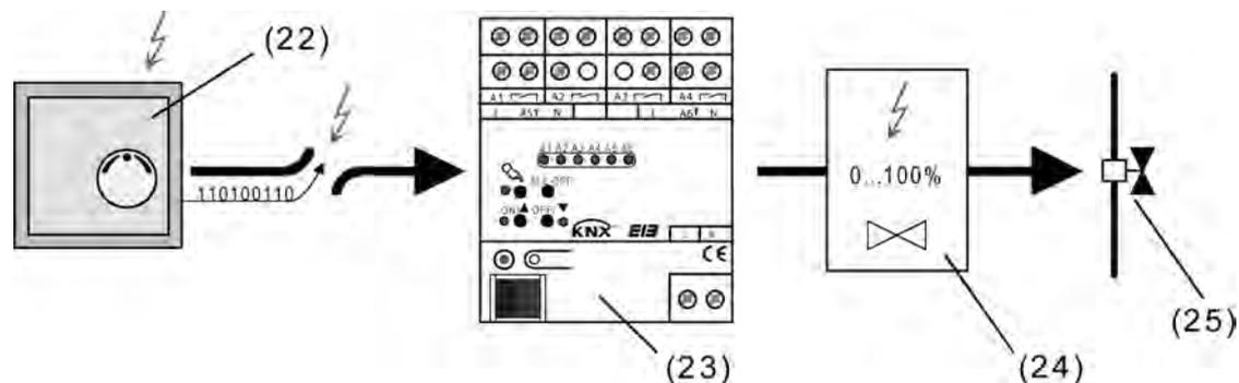
Figure 67: Principle of cyclical command value monitoring in the event of a fault (e.g. open circuit)
