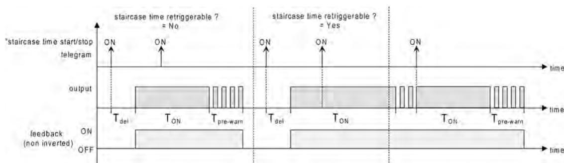
Figure 18: Switch-on behaviour of the staircase function
