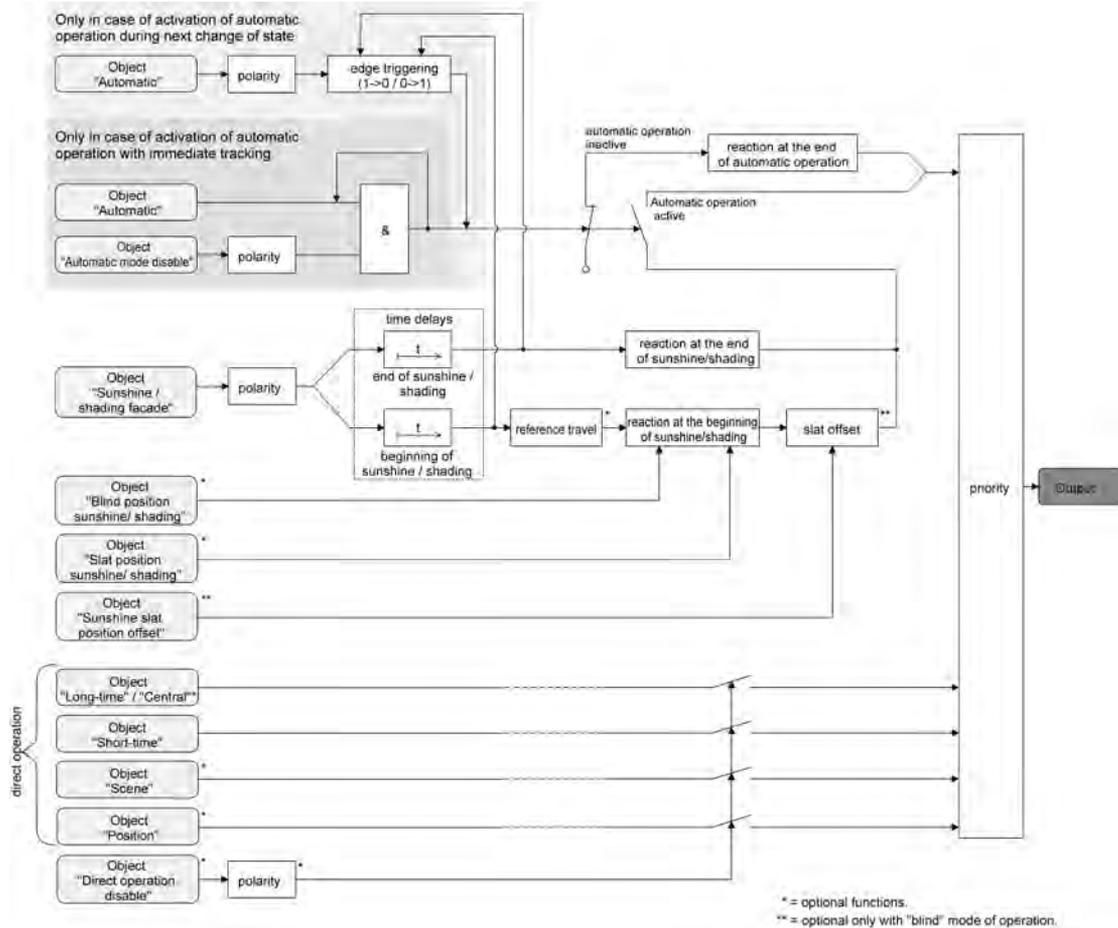
Figure 41: Function diagram illustrating the enlarged sun protection
