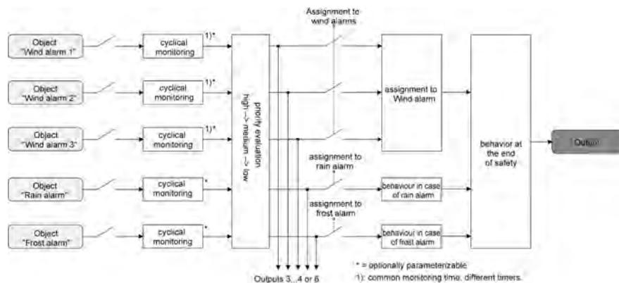
Figure 36: Function diagram of channel-oriented safety functions
