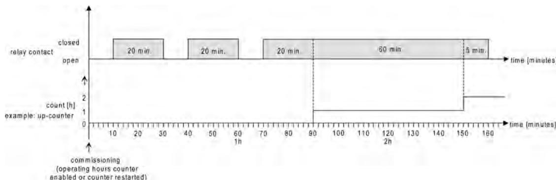
Figure 23: Functional principle of the operating hours counter
