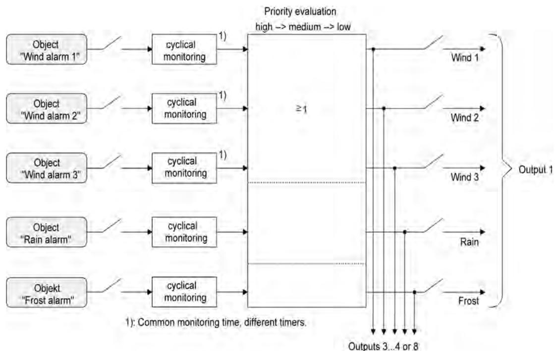
Figure 13: Function diagram of the safety function
