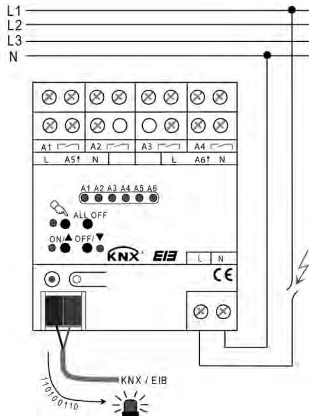
Figure 8: Monitoring of the mains voltage
