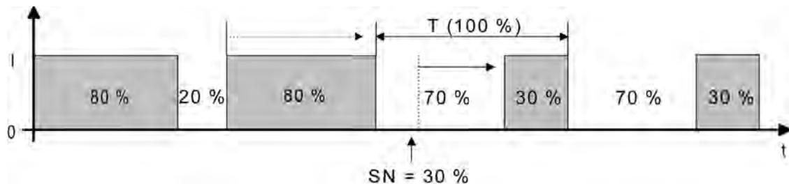
Figure 60: Command value change e.g. from 80 % to 30 % during the closing phase of the valve
