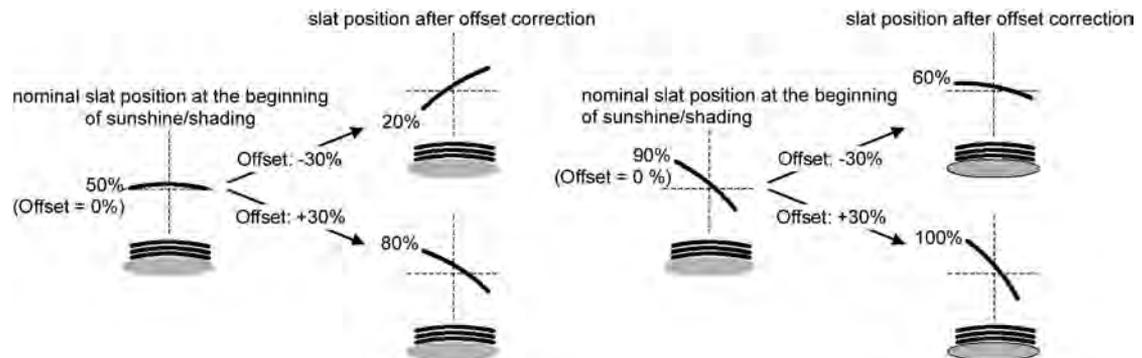
Figure 42: Functional principle of slat offset
