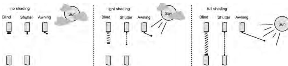
Figure 37: Sun protection principles (example)
