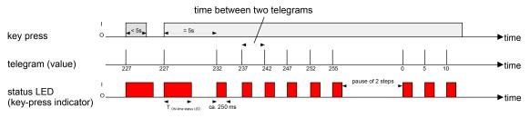
Image 9: Example of value adjustment with value range overflow
