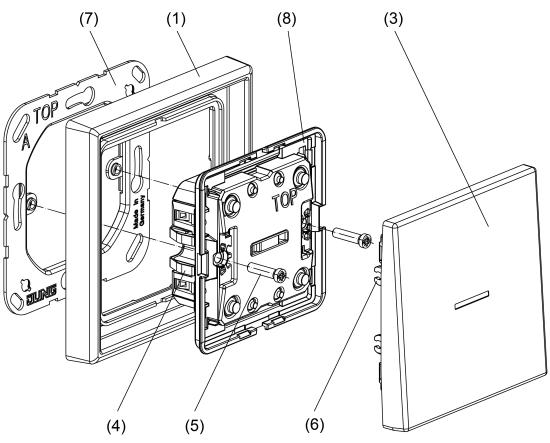
Image 3: Fitting the device
