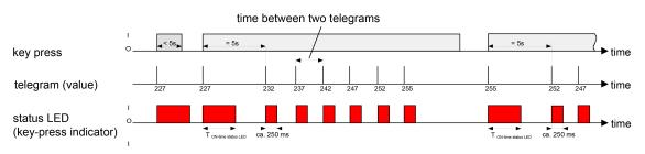
Image 8: Example of value adjustment without value range overflow
