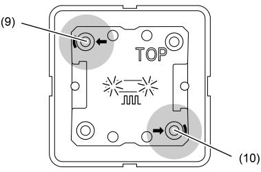
Image 6: Buttons for activating Programming mode
