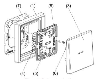
Figure 3: Fitting the device
