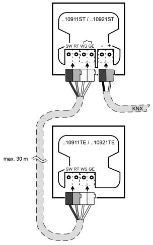
Figure 4: Connecting push-button extension
