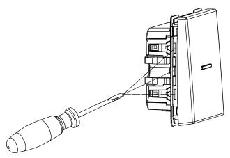
Figure 7: Dismantling rocker from the side
