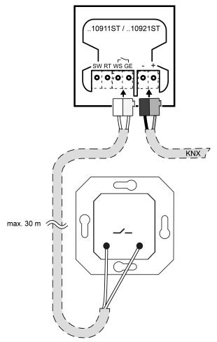
Figure 5: Connecting installation push-button
