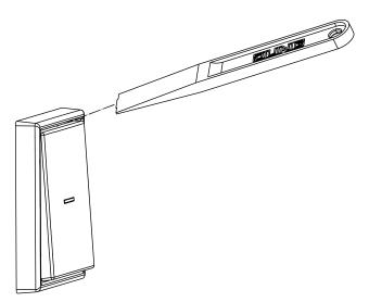
Figure 8: Dismantling rocker from above
