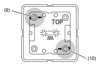
Figure 6: Buttons for activating Programming mode
