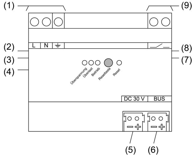
Figure 2: 1280 mA power supply – view
