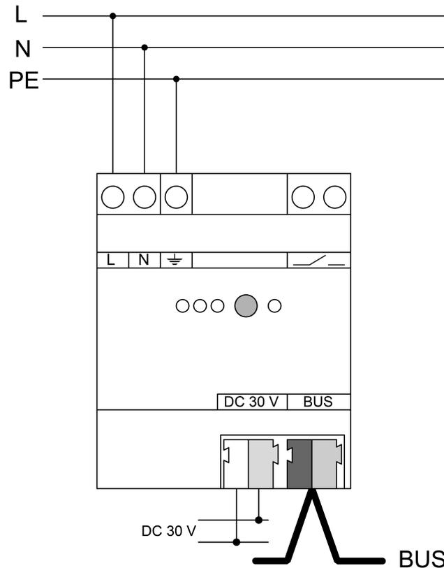
Figure 3: Wiring example – mains voltage and bus line
