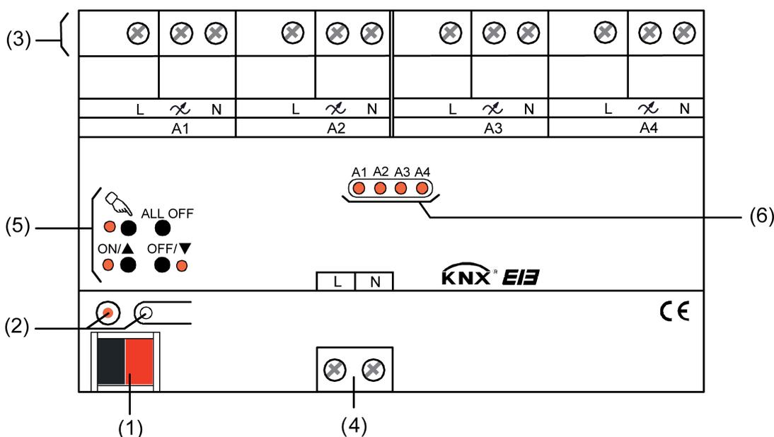
Figure 3: Structure of the 4-gang display variant
