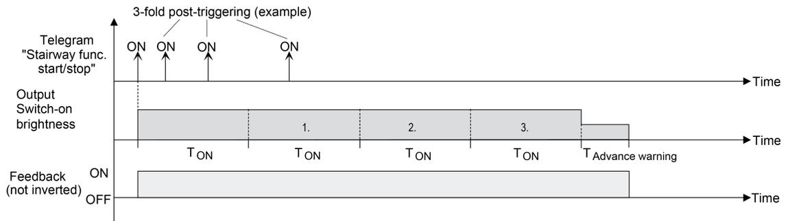
Figure 30: Time extension of the staircase function
