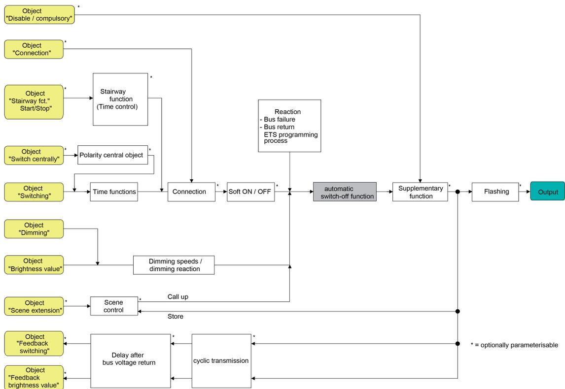
Figure 20: Function diagram of the automatic switch-off function
