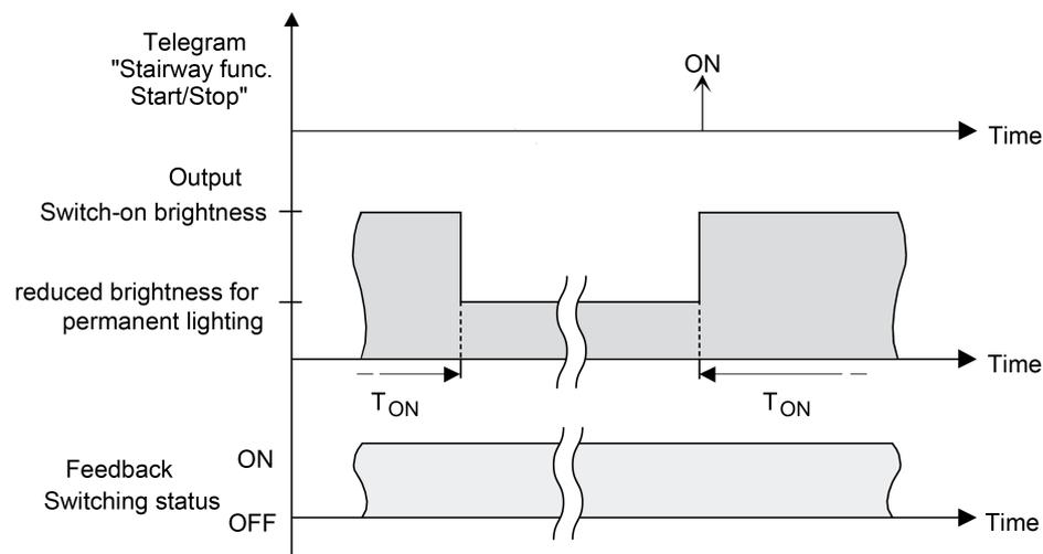
Figure 28: The continuous lighting of the staircase function without soft functions
