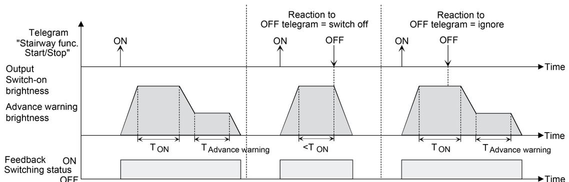
Figure 25: Switch-off behaviour of the staircase function with soft functions
