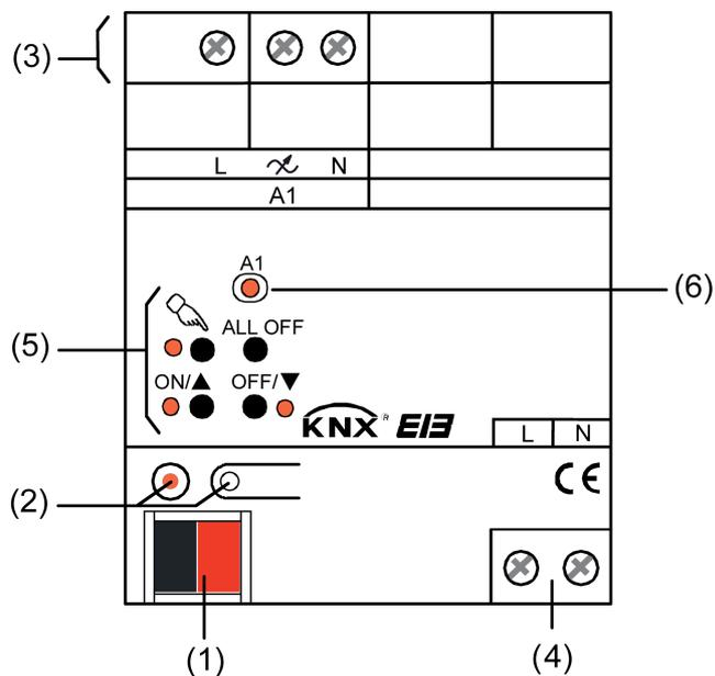
Figure 1: Structure of the 1-gang display variant
