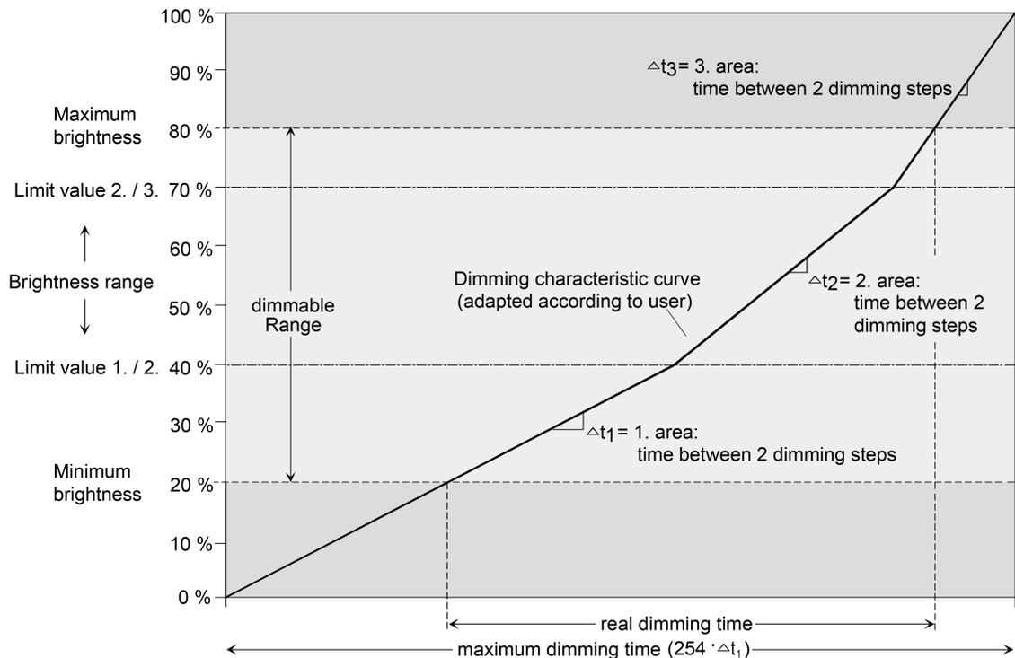
Figure 40: User-defined dimming characteristic as an example with minimum brightness and maximum brightness
