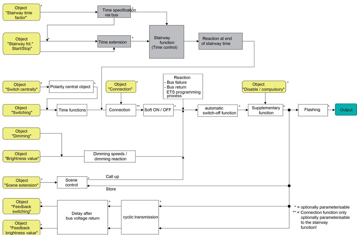
Figure 21: Function diagram of the staircase function
