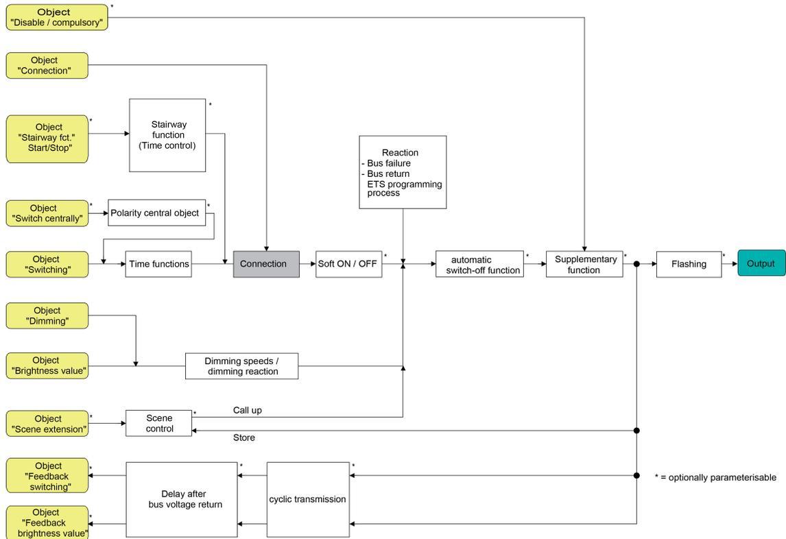
Figure 35: Function diagram of the logic operation function
