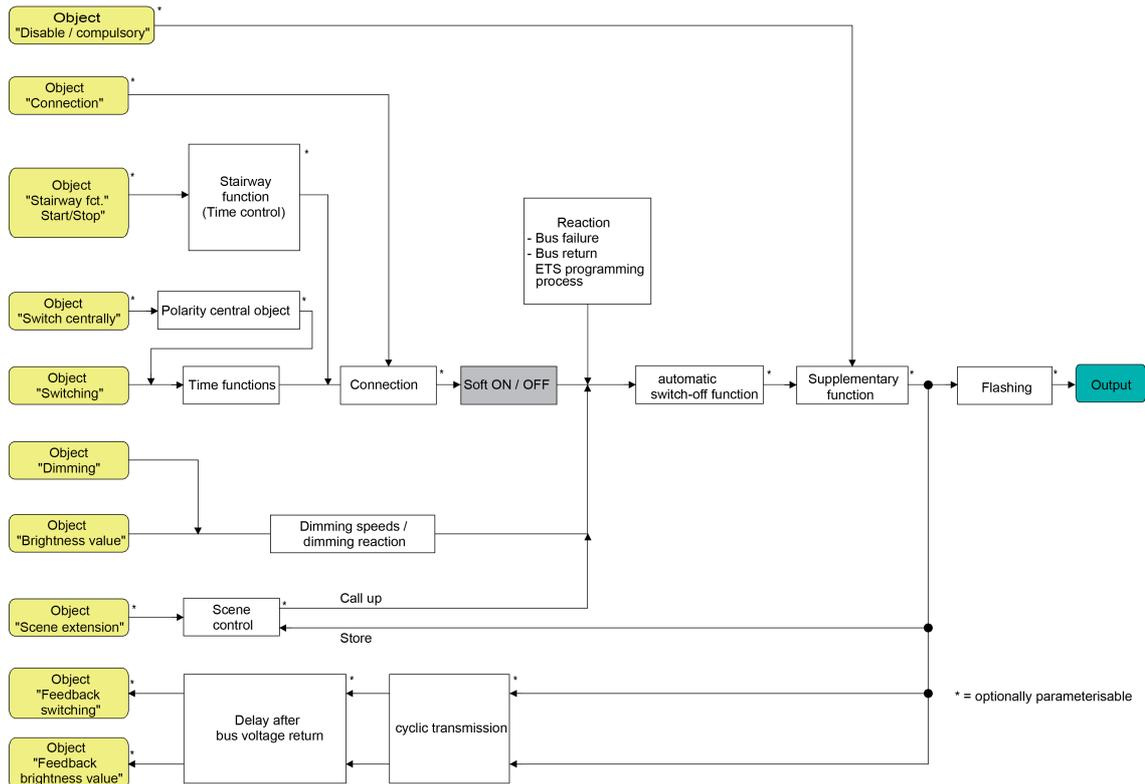
Figure 18: The function diagram of the soft functions
