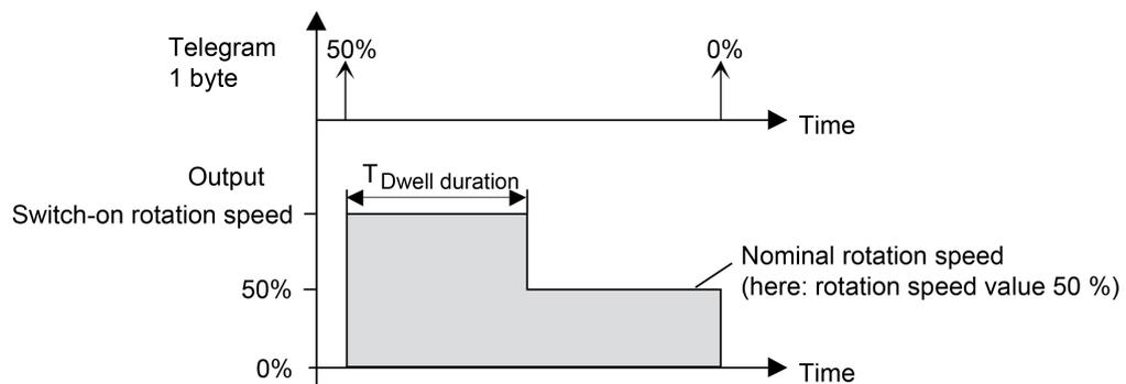
Figure 42: Cutting-in speed and required speed for value commands
