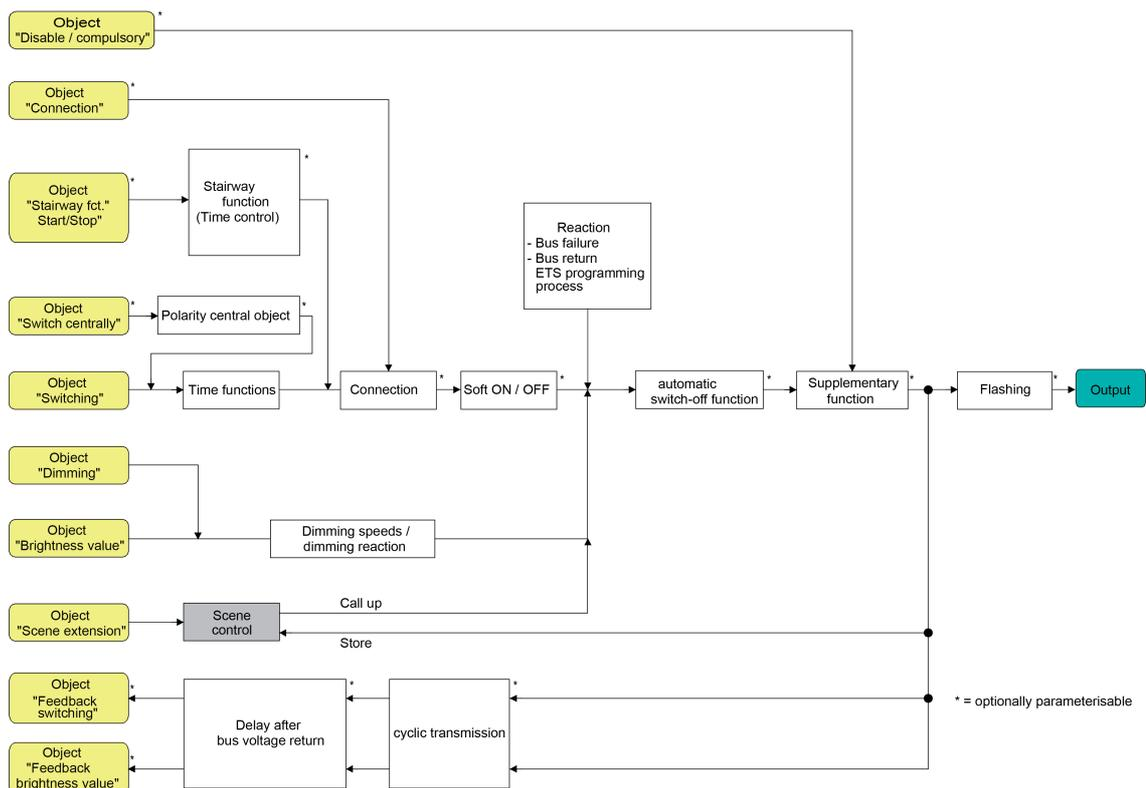
Figure 31: Function diagram of the scene function
