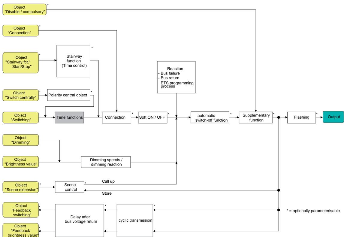
Figure 16: Function diagram of the timing functions
