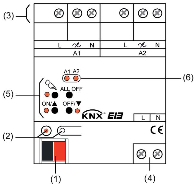
Figure 2: Structure of the 2-gang display variant
