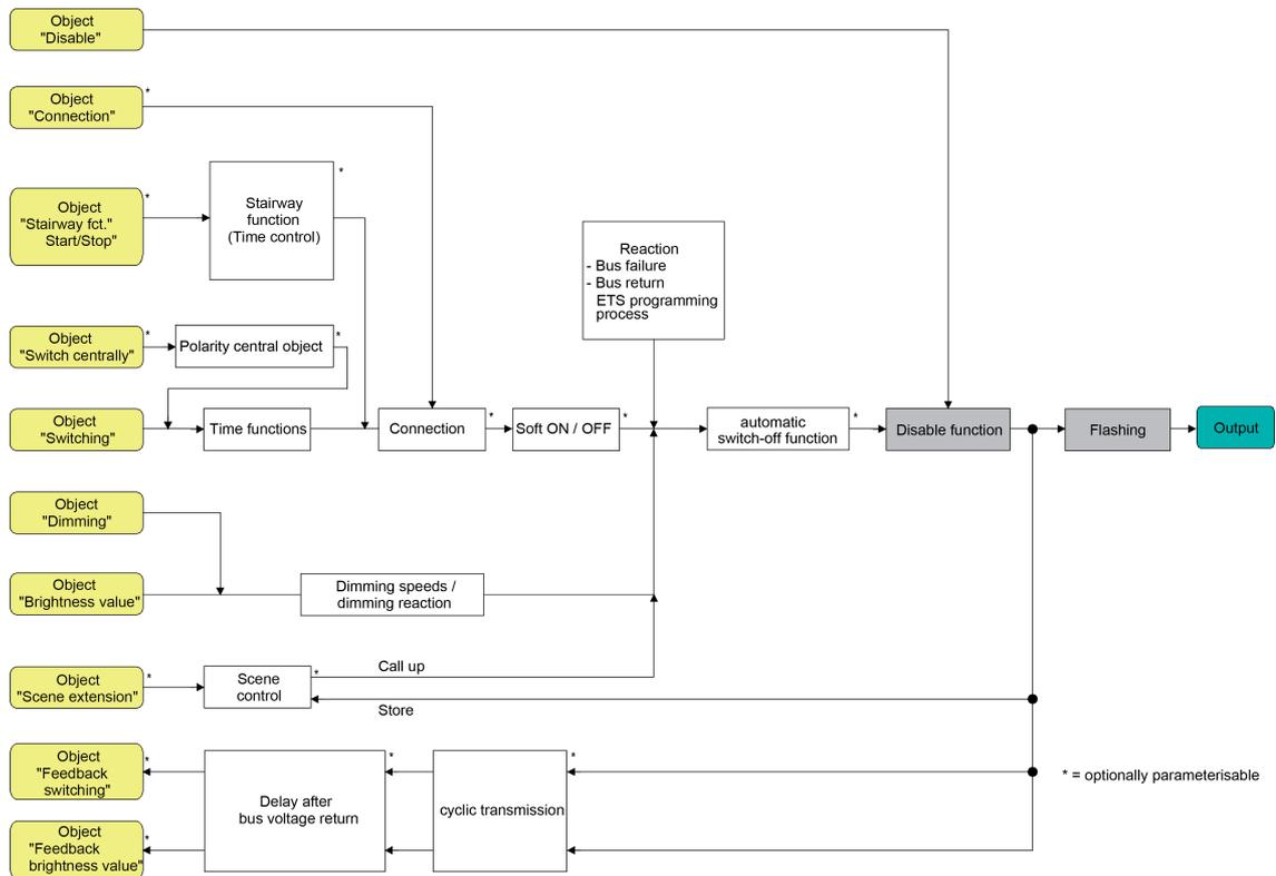
Figure 33: Function diagram of the disabling function
