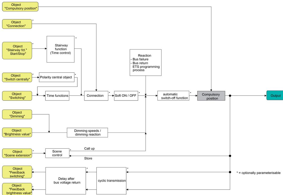
Figure 34: Function diagram of the forced position function
