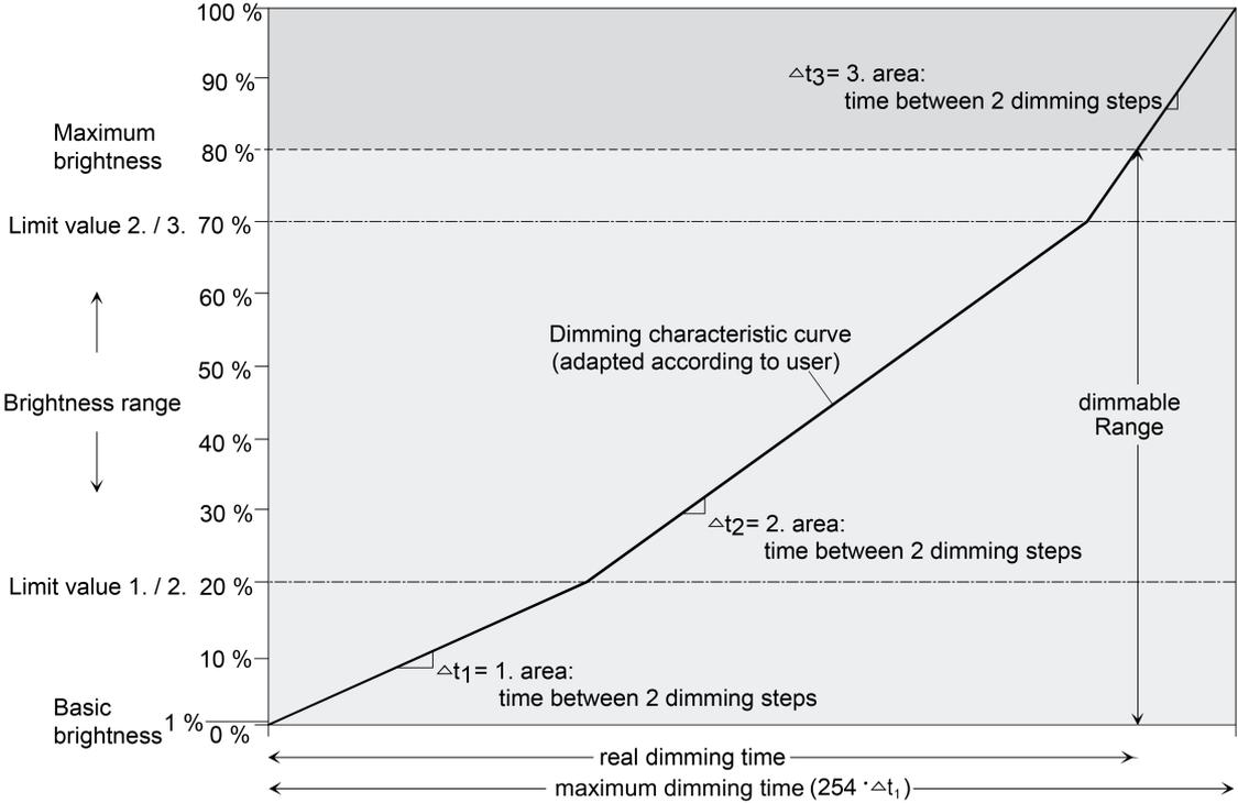
Figure 39: User-defined dimming characteristic as an example with basic brightness and maximum brightness
