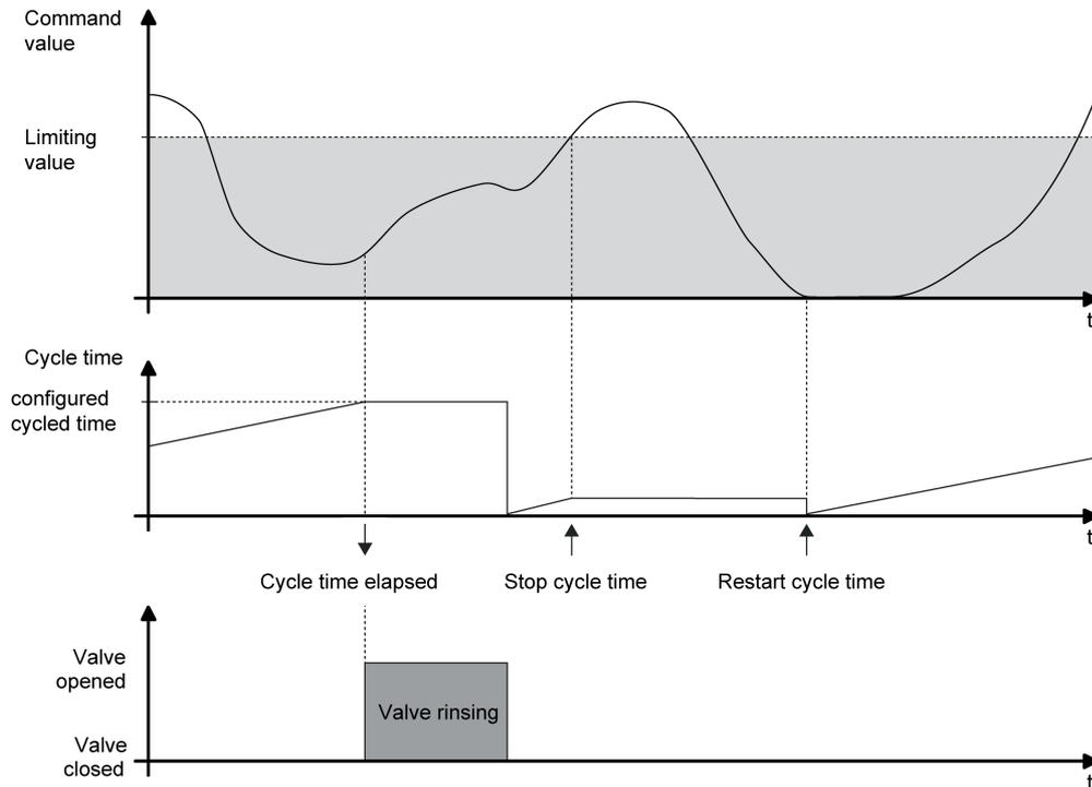
Figure 20: Example of a minimum command value limiting value for intelligent valve rinsing
