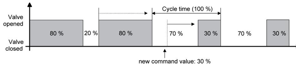
Figure 6: Example of a command value change 80 % -> 30 % during the closing phase of the valve
