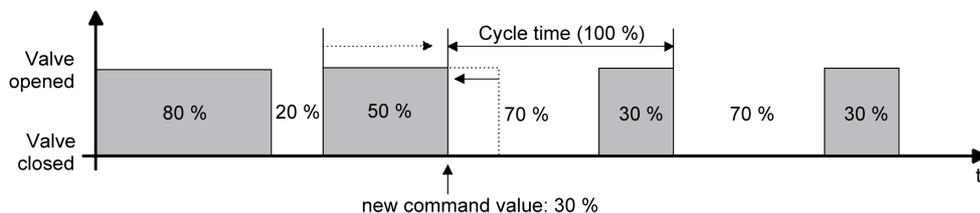
Figure 7: Example of a command value change 80 % -> 30 % during the opening phase of the valve (opening phase too long)
