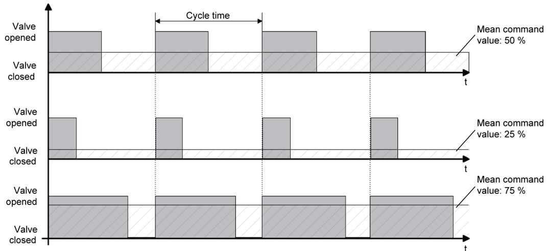
Figure 4: Resulting mean value through variable duty factor with pulse width modulation
