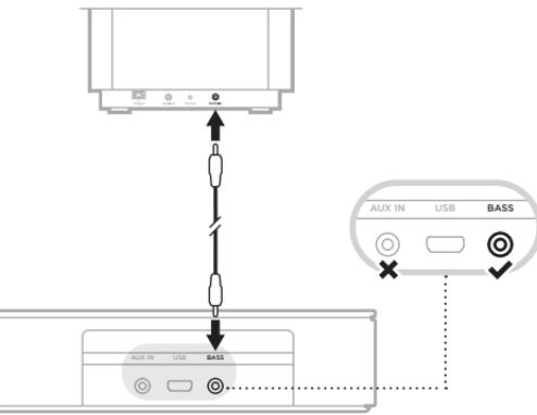
Connect a 3.5 mm audio cable (not provided) to the bass module's **BASS IN** connector and the speaker's **BASS** connector (not the **AUX IN** connector).
