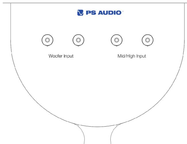
Note: Binding posts may have plugs. If using banana plugs, remove the plugs first.
