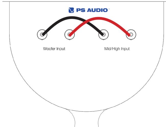
For bi-wiring/bi-amping do not connect the jumpers (as seen below).
